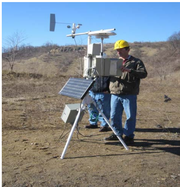
Figure 5-9: Monitoring station at a mine site
