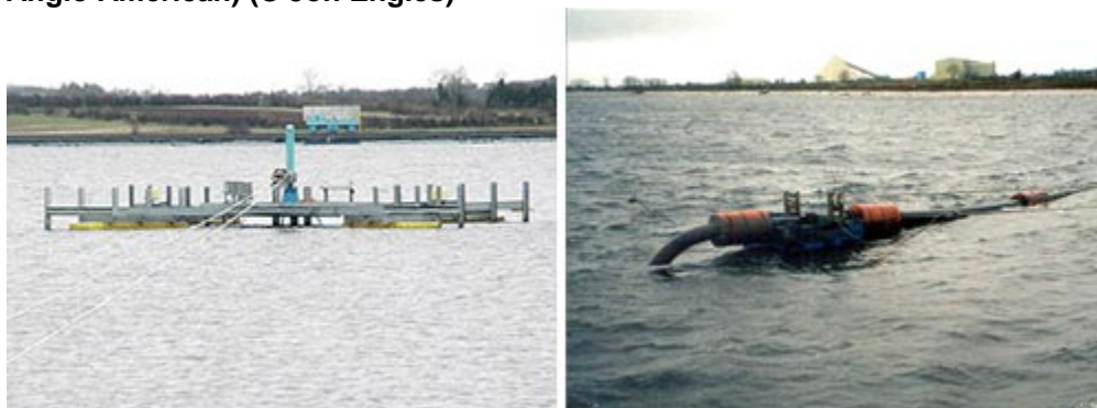
Figure 5-11: Subaqueous deposition within a conventional tailings impoundment (Courtesy Anglo American) (© Jon Engels)
