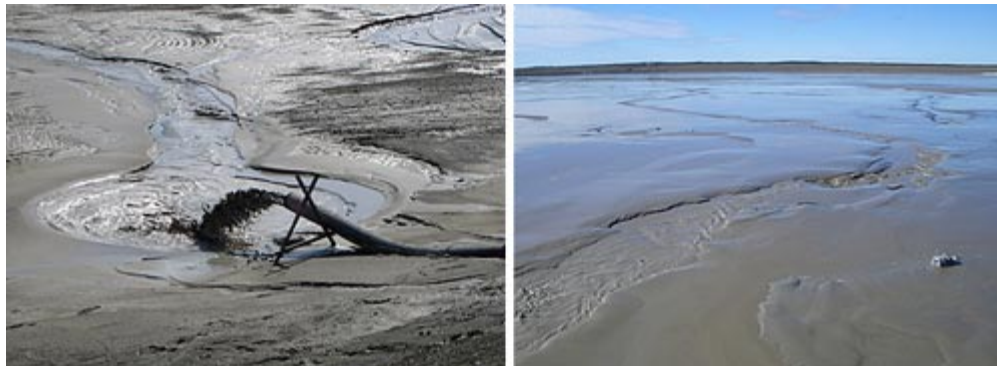
Figure 5-10: Sub aerial tailings discharge (left) and shallow low velocity braided streams on a tailings beach (right) (© Jon Engels)
