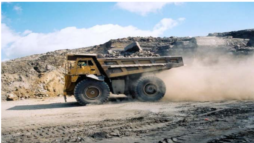
Figure 5-2: Road dust at a mining site
