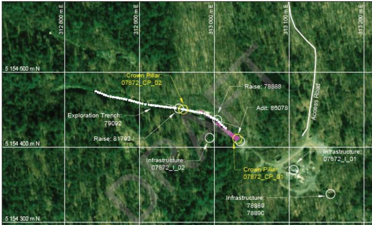
Figure 2 – Location of mine hazards proposed for rehabilitation. Image source: Golder Associates Ltd. (2021).
